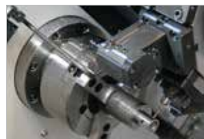
Chuck Air Blow (Upper Chuck)
