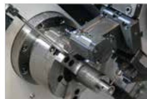
Chuck Air Blow (Upper Chuck)
